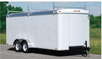
Atlas auto haulers are known for solid construction. These rounded top trailers are framed with steel tubing with 3/8" plywood lining. Other features are:
